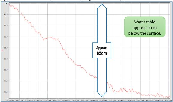
Fig 7. Groundwater level for Piezometer 9, high southern seep, Nov - Dec 2016
