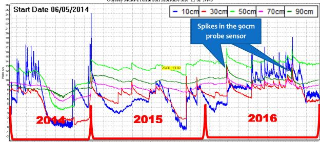
Fig 2. Soil moisture probe readings for non-wetting sandhill site, May 2014-Dec 2016
