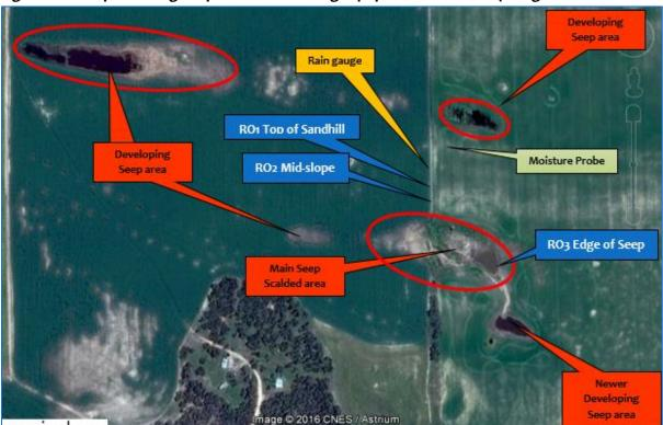
Fig 18. Site map showing seeps and monitoring equipment locations (Google Earth Oct 2016)
