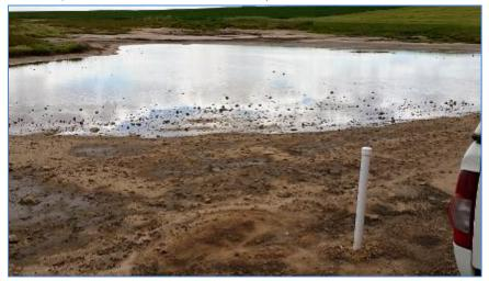
Photo 20. Main seep view from midslope piezometer Ro2.
