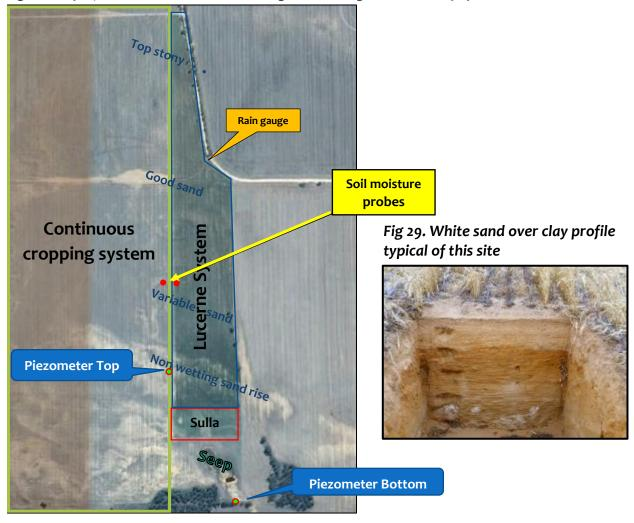
Fig 28. Map of Bond Lucerne Trial showing monitoring zones and equipment sites
